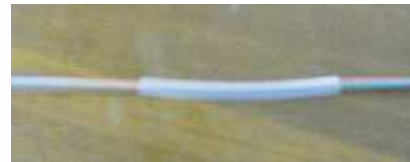
Pic 3:the length of stripped fiber cable Pic4: fiber after stripping Pic5: use EVA transparent tube to protect the stripped fiber
